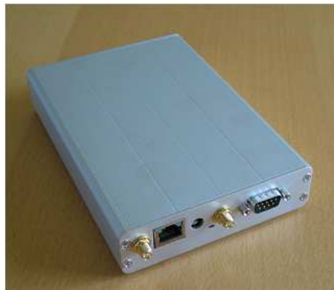
Figure 13: 4G Cube – compact wireless router
