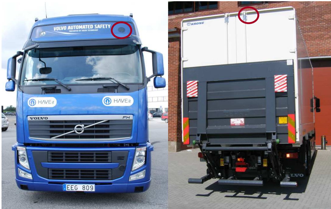
Figure 2: Integration of the V2V units on the AQUA truck.
