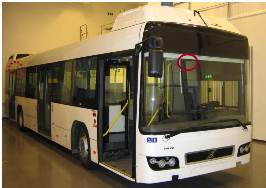
Figure 3: Mounting locations for the V2V units on the WP5400 bus.
