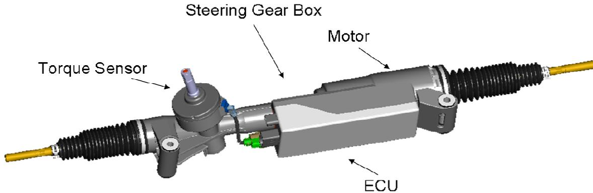
**Schematic view of the electric steering actuator**
