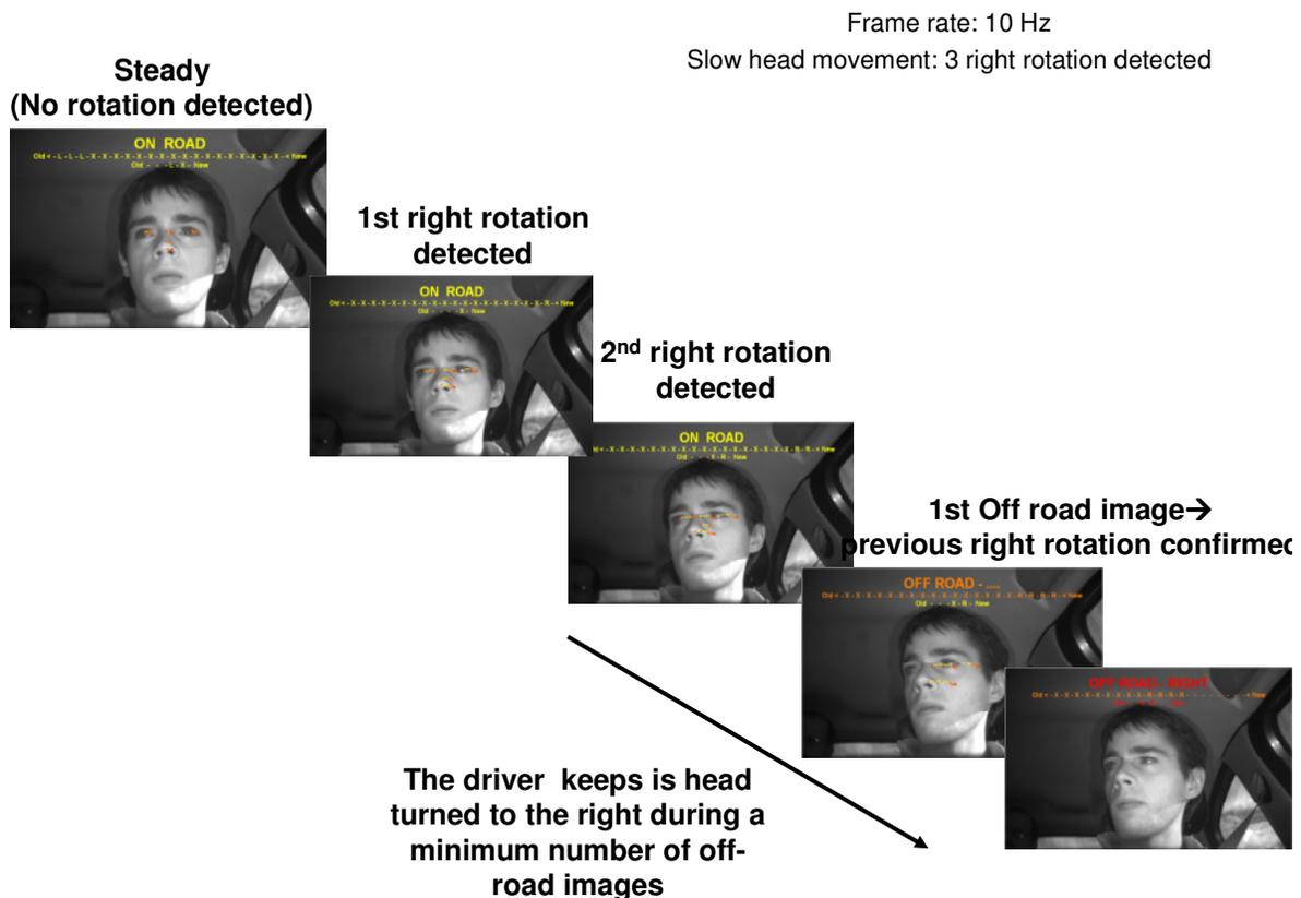
Figure 10: Typical sequence of head rotation detection and classification
