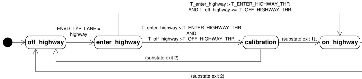
Figure 2: Top-level state chart of the DSA module
