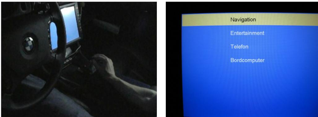
Figure 7: Display of secondary task presentation in the middle console with joystick (left) and contents of the hierarchical menu (right).
