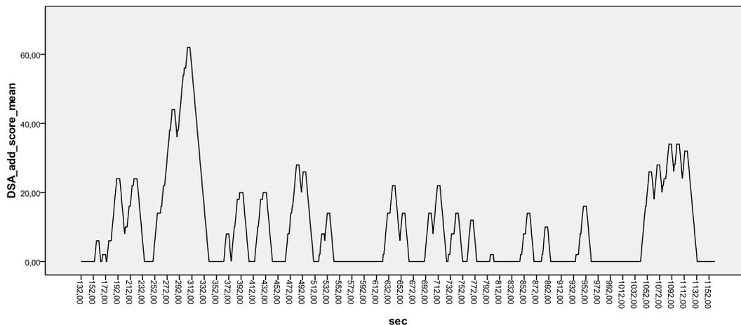
Figure 9: Internal signal SCORE\_ADD over a 20 minutes baseline drive with the performance of a secondary task for Driver D03.
