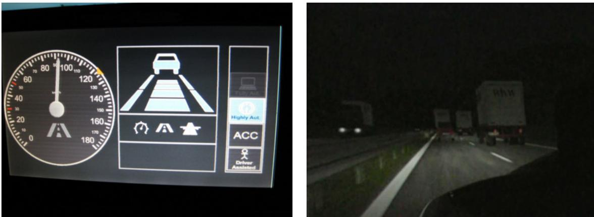
Figure 5: The HMI of the HAVEit system showing the state “Highly Automated mode” (left) and one of the night-time scenarios “traffic jam” (right) in the validation study.
