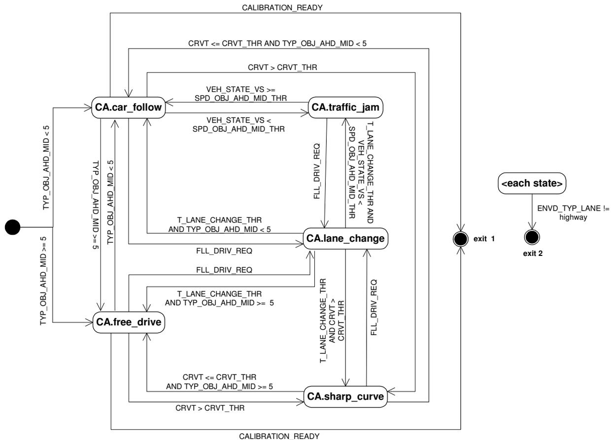
Figure 4: Substates of top-level state "calibration"
