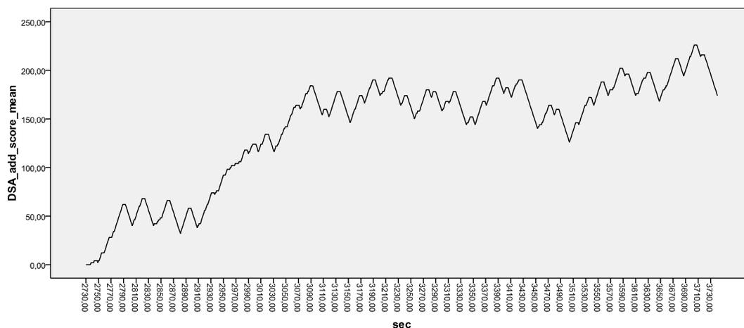
Figure 8: Internal signal `SCORE_ADD` over a 20 minutes baseline drive with the performance of a secondary task for Driver D02
