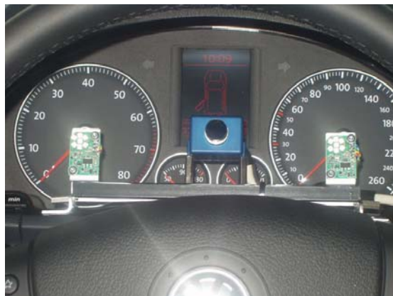
CAF Camera integrated into VW Golf V
